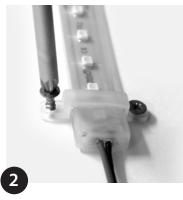
Place strip in clips and fix remaining screw. Do not over tighten.
