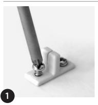
Fix clips with suitable screws (min. 5 clips per metre or every 250mm/9.84").
